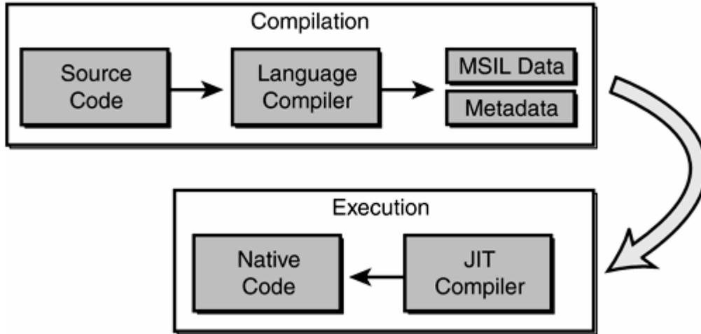
The runtime includes a feature called just-in-time (JIT) compilation that translates the MSIL code into the machine language (Native Code) of the system on which the application will run. When a client device on the .NET platform launches the Visual Basic .NET application, it starts running in the machine language of the client system and can fully integrate and interact with other .NET-based applications and services regardless of the language in which it was developed.
