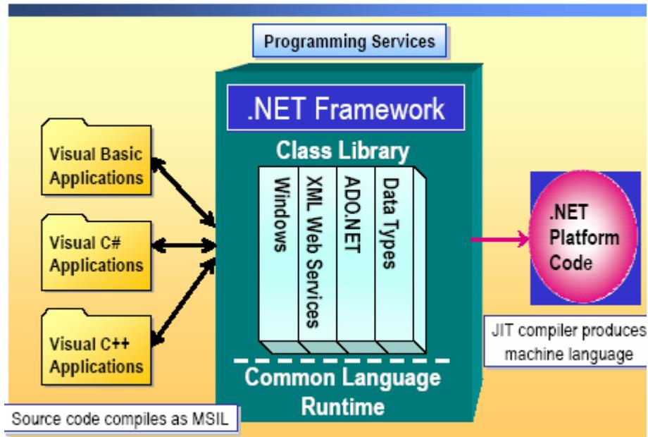
**The .NET Framework** is a set of programming services designed to simplify application development in the highly distributed environment of the Internet. The .NET Framework has two main components: the common language runtime and the class library.
